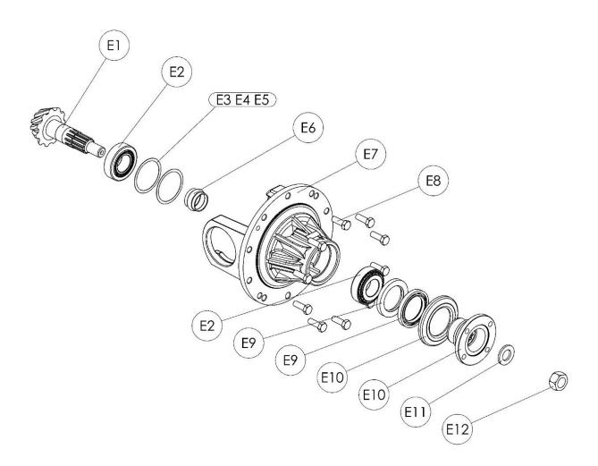
Section 'B' - Main Case and Differential Assembly
